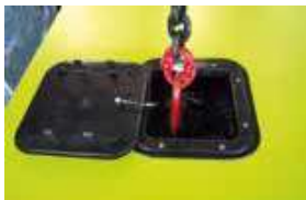
Integrated central lifting point
