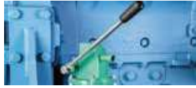
Manual lube oil drain pump
