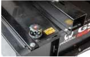
Integrated metal fuel tank
