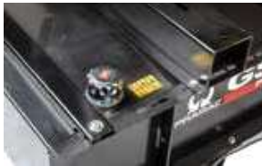
Integrated metal fuel tank
